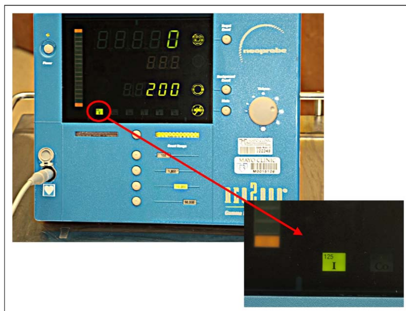
Figure 3 Gamma probe settings to detect ^{125}\text{I} for intraoperative localization of the radioactive seed.
