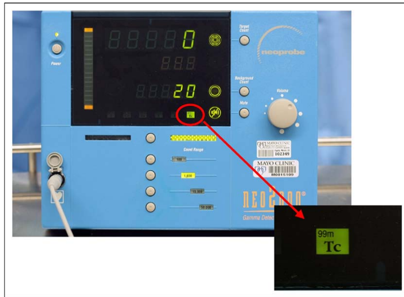
Figure 2 Gamma probe settings to detect ^{99m}\text{Tc} for SLN identification.
