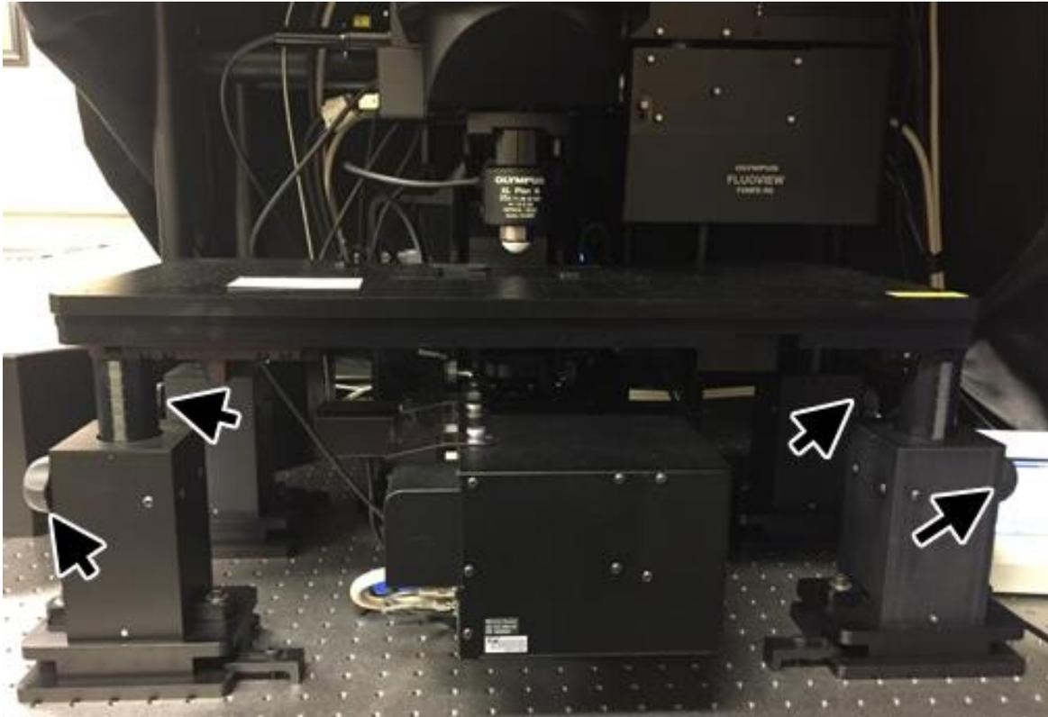
2. Depending on the objective and your sample size, you may need to adjust the height of the stage in order to have enough space between them. Touch the **upper arrow head** on the microscope control panel to raise the objective.
