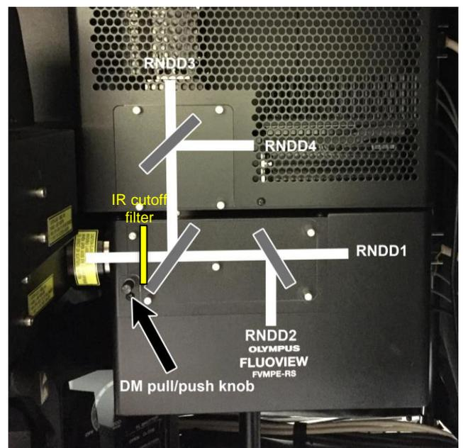
To check the current setting of dichroic mirrors and emission filters, use menu command, **Tool Window/Lightpath**.
