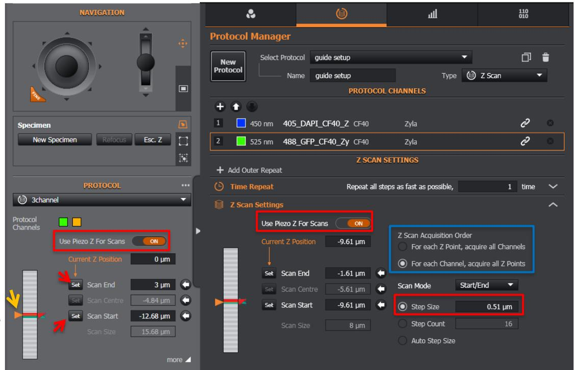
Type the **Step Size**, which represents focus movement in  $\mu\text{m}$ .
