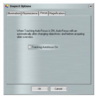
Figure 5.7: Tracking autofocus in the Inspect Options dialog box.
