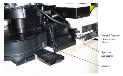
Figure 5.8: Fluorescence Components
