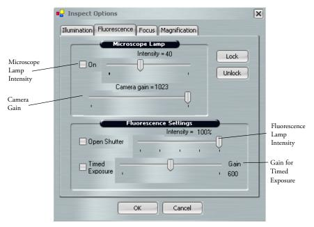
Figure 5.9: Fluorescence Tab in Inspect Options dialog box
