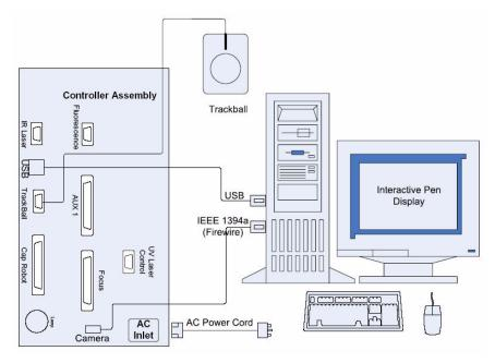
Figure D.1: Connections between the components of the Arcturus<sup>XT™</sup> Microdissection Instrument.
