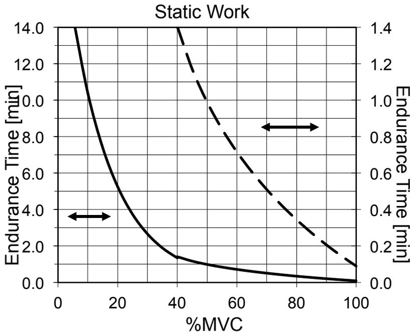
Note: There is a 4% (0.06 min, 4 s) discontinuity at 40 %MVC between the two equations.
